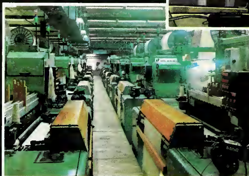
Van de Wiele Plush Weaving Machines —Weave apparel, upholstery, and carpets. Compact, high-speed machines guarantee high productivity.
